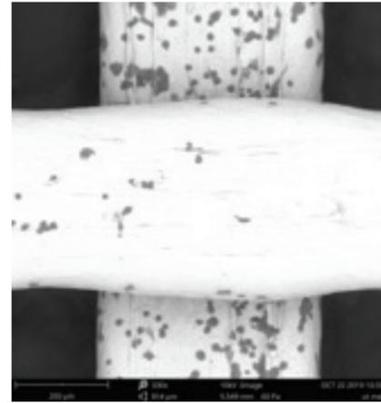
**Figure 2:** A PEEK bone scaffold using FDM 3D printing, covered with mineralised bone cells.
