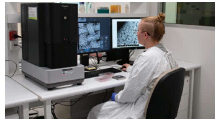
Phenom XL G2 desktop scanning electron microscope (SEM) at VectorLAB.
