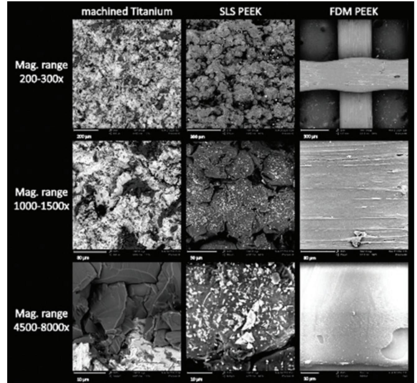
**Figure 3:** Visual summary of three possible bone implant materials. From the left, these are machined titanium, SLS printed PEEK and FDM printed PEEK. Note the difference in surface roughness which may affect the way the patient's bone cells will react to the surface.
