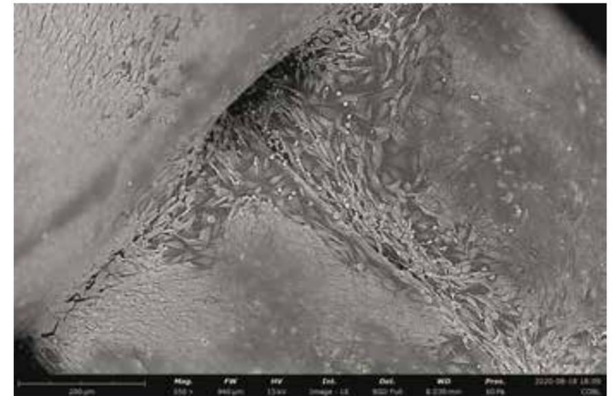
Low vacuum backscatter image of osteoblasts [bone cells] growing on the surface of the 3D printed scaffold. Images taken using the Phenom XL G2 desktop SEM.
