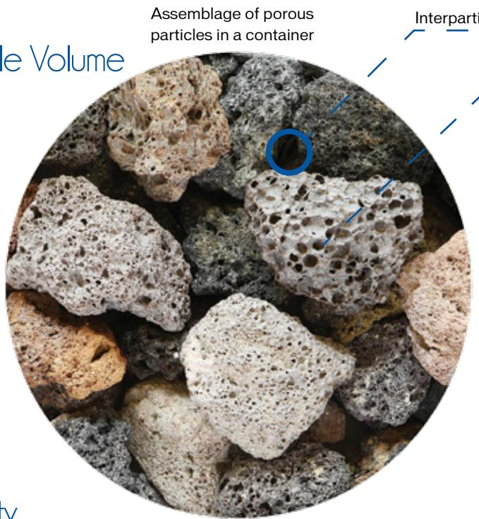
A single particle containing open and closed pores
