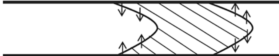
Figure 2: The role of radial diffusion The directions of the radial diffusion of the solute molecules are highlighted in Figure 2. At the front end of the pulse, the solute concentration is higher at the centre of the cylinder than at the cylinder walls. Hence, the solute molecules diffuse radially toward the cylinder walls. Since the solute molecules at the centre are travelling much faster than the molecules at the walls, the average axial velocities of these molecules are reduced by the diffusion. At the rear end of the pulse, the solute concentration is higher at the walls than at the centre, so the molecules diffuse radially toward the centre. This results in an increase in the average axial velocities of the diffusing solute molecules. Overall, the effect of radial diffusion is to slow the leading interface and accelerate the trailing interface thereby keeping the solute distribution more compact in the axial direction than it would have been under convection alone. The axial spreading due to the combination of both radial diffusion and convection ultimately results in the injected solute pulse developing a symmetrical concentration distribution, and is known as Taylor Dispersion .
