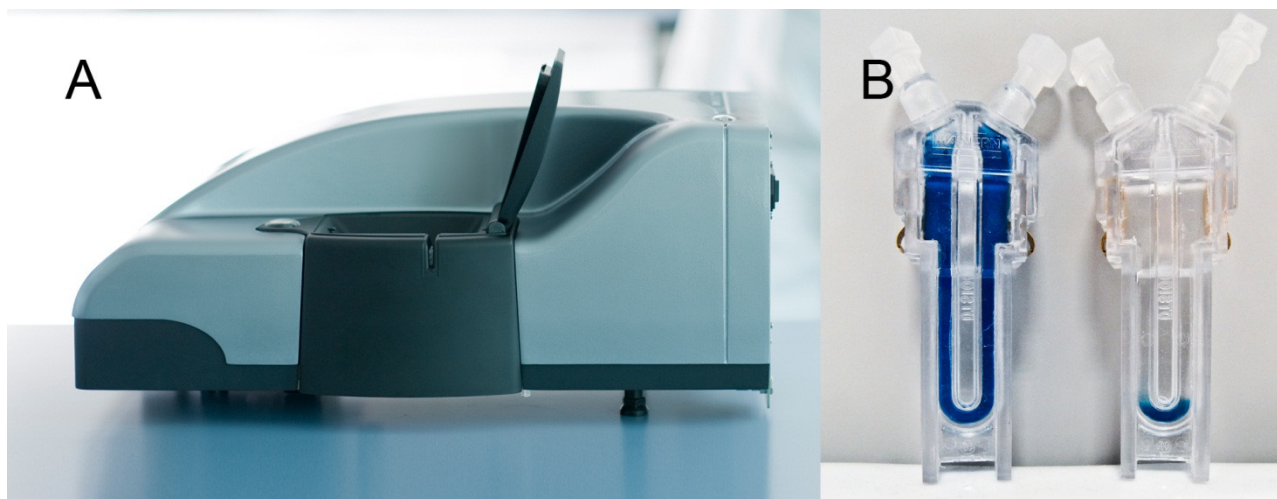
Figure 1: A. The Zetasizer Nano ZSP. B. Disposable folded capillary cells used for the diffusion barrier method.
