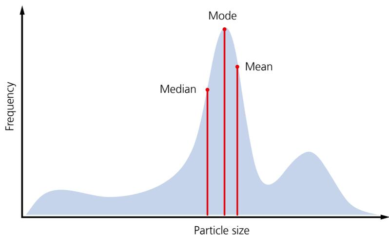
Illustration of the median mode and mean for a particle size distribution.
