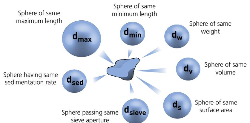
Illustration of the concept of equivalent spheres.
