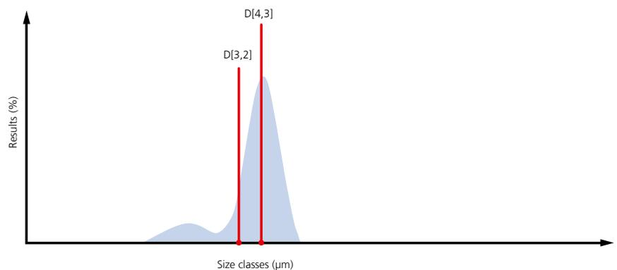
Illustration of the  $D[4,3]$  and  $D[3,2]$  on a particle size distribution where a significant proportion of fines are present.
