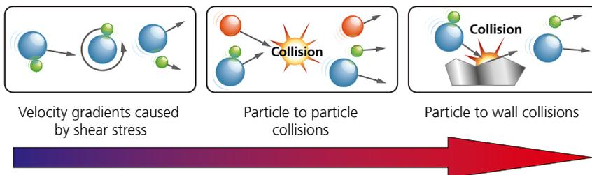
Illustration of the three dry powder dispersion mechanisms with increasing energy/ aggressivity.
