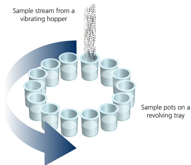
Illustration of a spinning riffler device.
