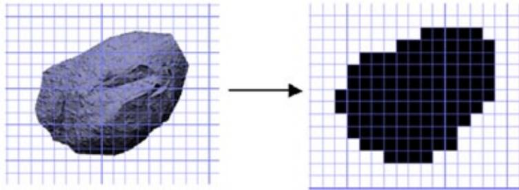
Conversion of a particle image into a 2D binary projection for shape analysis.
