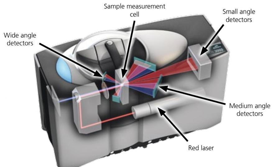
Optical layout of a state-of-the-art laser diffraction instrument.
