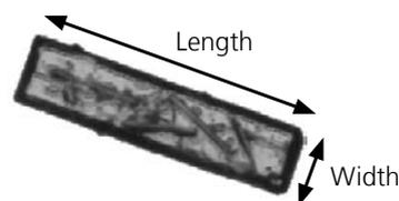
Illustration of length and width on a needle shaped particle image.
