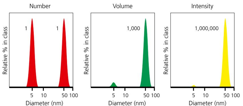
Example of number, volume and intensity weighted particle size distributions for the same sample.
