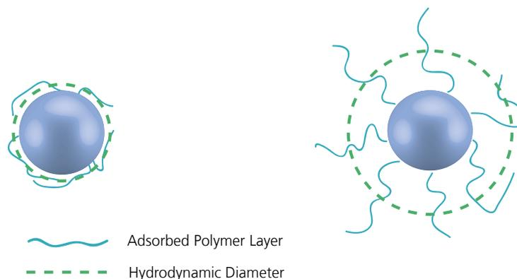
Illustration of the reported hydrodynamic diameter in DLS being larger than the 'core' diameter.
