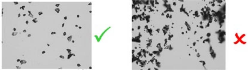
Illustration of the importance of sample dispersion for automated particle imaging.
