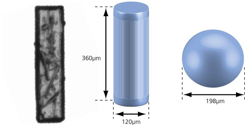
Illustration of the volume equivalent rod and sphere of a needle shaped particle.
