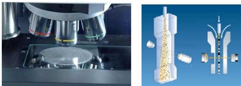
Illustration of static imaging (left) and dynamic imaging (right) optical arrangements.
