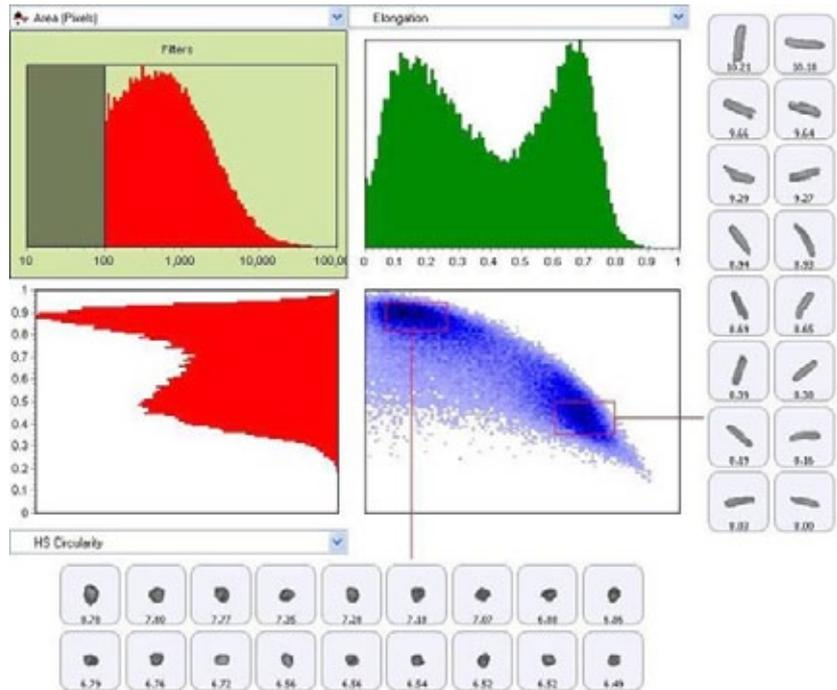
Use of scattergram tool to show classification of the sample by both size (elongation) and shape (HS Circularity).
