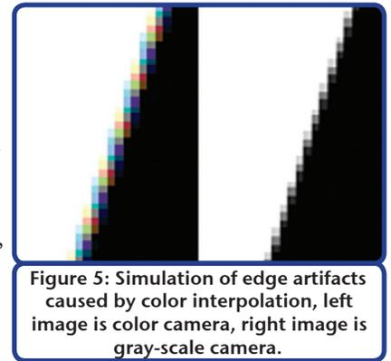
Figure 5: Simulation of edge artifacts caused by color interpolation, left image is color camera, right image is gray-scale camera.
