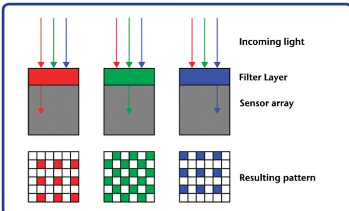
Figure 3: Cross-Section of Bayer color filter array (CFA) arrangement and resulting pattern on monochrome sensor.
