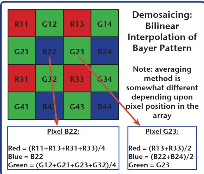
Figure 4: Demosaicing of Bayer color filter array (CFA) showing resulting RGB pixel values created using bilinear interpolation.
