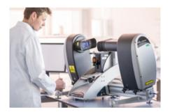
Run the measurement by selecting the desired SOP from the menu system. This automatically configures the system and ensures everything is optimally set to deliver accurate results, including auto-alignment of the optical system. Synchronization of external systems such as extractors, actuators and positioning systems is also supported.
