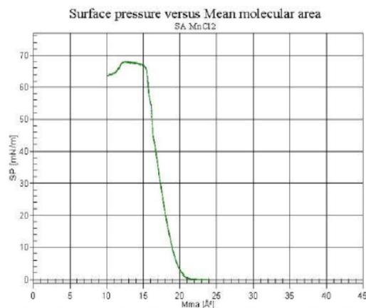
Screen shoot KSV NIMA LB software; Surface pressure against mean molecular area for steric acid in water - MnCl<sub>2</sub>
