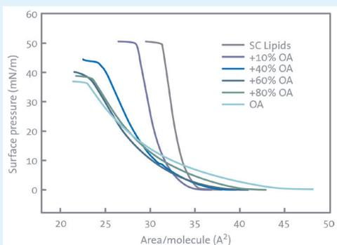
THE ISOTHERMS OF MODEL SKIN LIPIDS WITH INCREASING LEVELS OF OLEIC ACID. With permission from Langmuir 2013, 29 (15), pp 4857–4865. Copyright 2013 American Chemical Society.
